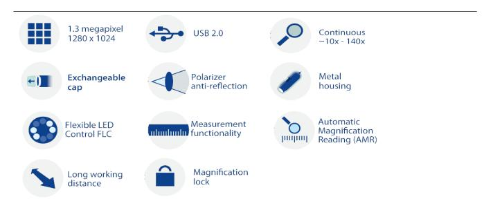
The AMR function automatically detects and displays the magnification of the Dino-Lite. The magnification is displayed within the Dino-Lite software and stored with the captured picture and simplifies the measuring process. Because of the built-in polarization filter this model is ideal when working with shiny or reflective objects such as metal, plastic, glass, jewelry, electronics, etc.
